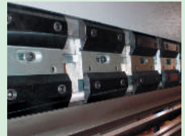
Quick top tool clamping system by Amada Promecam to change the tools easily
