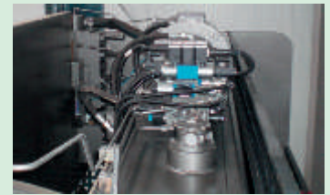
Hydraulic system made by Rexroth which supply oil flow to cylinders proportional
