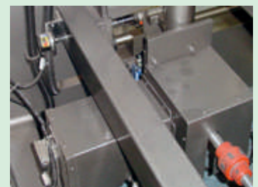
Backgauge system by Unimec driven by AC servo motors with 0,01 tolerances.
